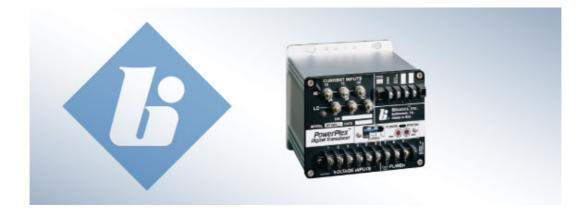
The PowerPlex® instrument is a utility-grade, three-phase, digital power transducer that connects directly to instrument transformers. Direct-connect high-voltage inputs are also available. The design and components are field-proven in the substation environment with all inputs transformer isolated.
